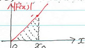
$$\begin{aligned}W &= \frac{1}{2} \times kx_0 \cdot x_0 \\ &= \frac{1}{2}kx_0^2\end{aligned}$$
