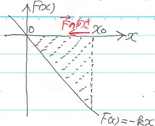
$$\begin{aligned} \text{仕事 } W &= \int_{x_0}^0 F(x) dx \\ &= - \int_{x_0}^0 kx dx = -k \left[ \frac{x^2}{2} \right]_{x=x_0}^{x=0} \\ &= +\frac{1}{2} k x_0^2 \end{aligned}$$
