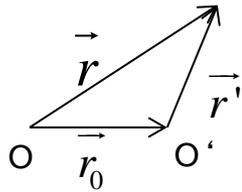
$$\vec{r} = \vec{r}_0 + \vec{r}', \vec{\ell} \equiv \vec{r} \times (m\vec{v}), \vec{\ell}' \equiv \vec{r}' \times (m\vec{v}),$$
